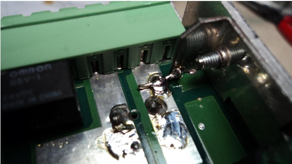
This made a very big difference. I then bypassed the +28 V and +21V terminals on the circuit board with 1  $\mu$ F ceramic capacitors. Power supply noise is now almost completely inaudible on any frequency within the receiver's range.
