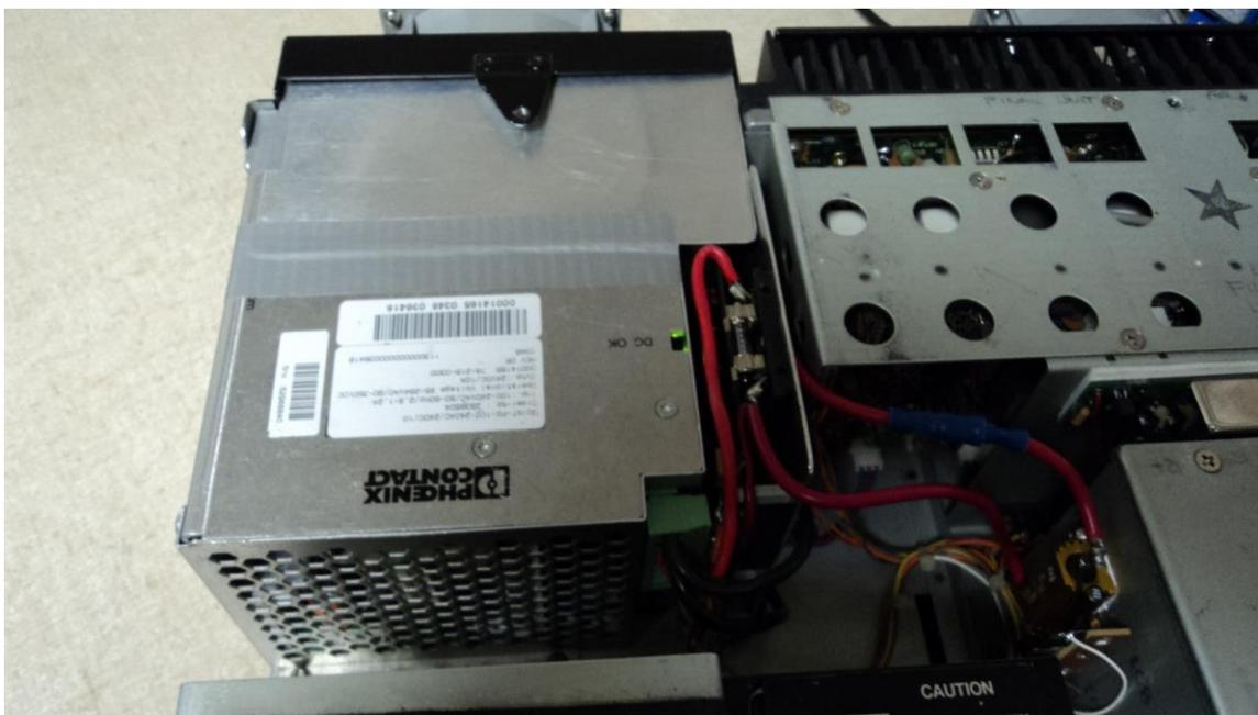
The rear case-half attachment screws on the left-hand side must be shortened by 2mm in order to avoid bottoming out against the case of the Quint.
