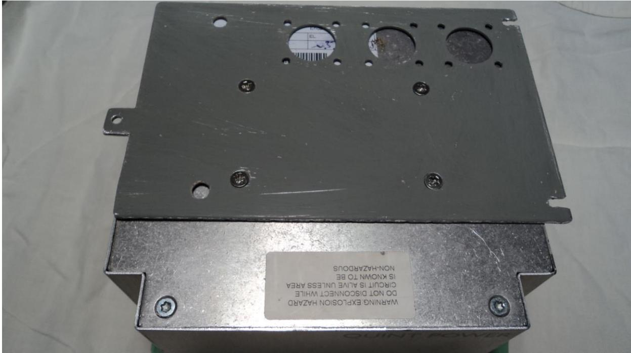
The original case-mounting bracket on the left-rear of the chassis has to be modified slightly so as to clear two of the Quint case screws. See Photo 2.
