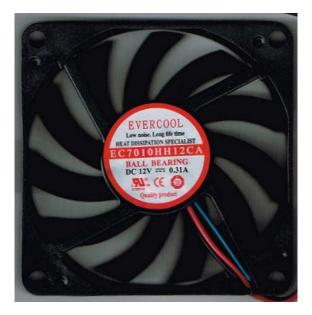
This is a 70mm x 70mm x 10mm slim ball-bearing fan. It's a three-wire design but you can just re-pin your 2-pin connector to use the red and black leads or keep your Kenwood pigtail and wire it to the red and black leads at the fan. If you use this fan, it will be completely contained within the OEM fan housing, and you can put the Quint right up against the housing. Your Quint and the radio will run STONE cold.
