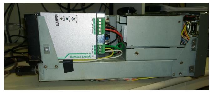
There's actually a method to my madness. Once you re-install the lower case of your radio, it will be easy to reach the terminals and the voltage adjustment screw if necessary. The new AVR board supplied with Jeff's kit has supply wires that easily reach the DC output terminals, and this setup places the Quint's intake and cooling fins directly in the PS fan's airflow. Plus, I think it makes the installation look factory.
