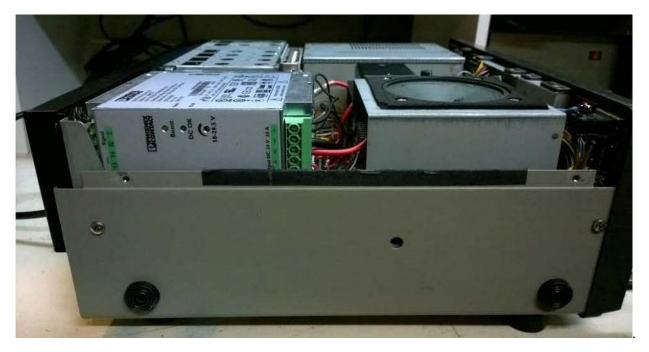
I use an Evercool 70mm x 70mm x 10mm ball-bearing muffin fan for the PS which is a good substitute for the stock fan. It has the same approximate current draw, and it uses the same holes too. More info can be found in the APPENDIX.
